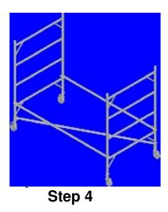
Install 4 diagonal braces (silver) inside frame from bottom transom to third transom up (2spaces). These should be as close as practical towards the outside of the frame. Level scaffold in each direction using height adjustable screws jacks.
