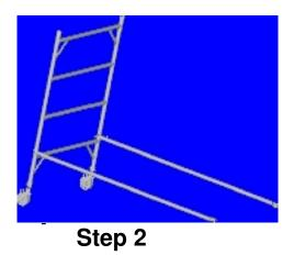
Lock brakes on castors of second base frame and attach horizontal braces to INSIDE of standards. Use screw jacks to approximately level scaffold. Ensure tommy bars on castors are pushed in to prevent injury.
