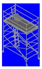
Please note that when horizontals are clipped to standards (vertical component) they are designed for sideways deflection only and are not load supporting. Therefore do not step on these horizontals when climbing the scaffold. Do not stand on midrails and handrails.
